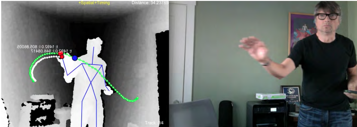
Figure 1: Captured motion is reproduced using our sonification as a learning aid with our system, SoundTracer
