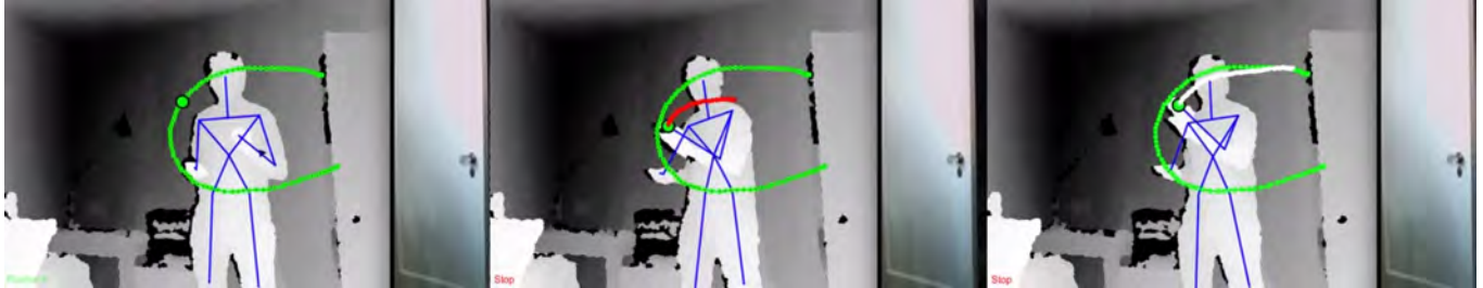
Figure 2: Student attempting to reproduce motion path. Student's path turns white as it approaches the reference path.
