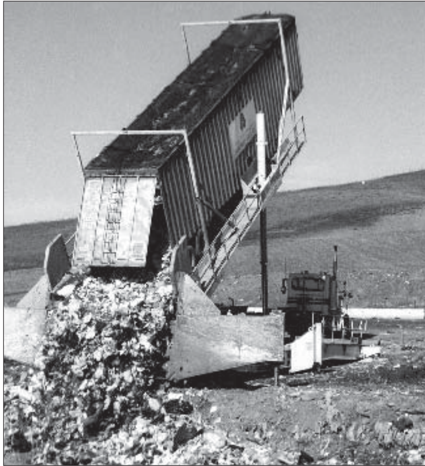
These trucks transport 2,600 tons of solid waste produced in San Francisco per day to the landfill. Each truck holds about 26 tons, and each of the 30 trucks in the fleet makes an average of 3 trips a day.
