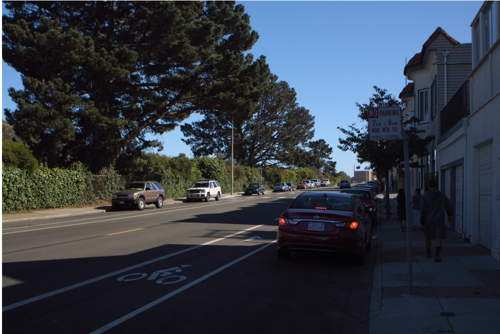
Figure 5: A Class II Bicycle Facility on San Bruno Avenue, part of Bicycle Route 25. Author Photo.
