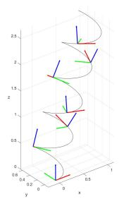
Figure 1: Circular helix with its Frenet frame. The tangent vector is red, the principal normal vector is green, and the binormal vector is blue.
