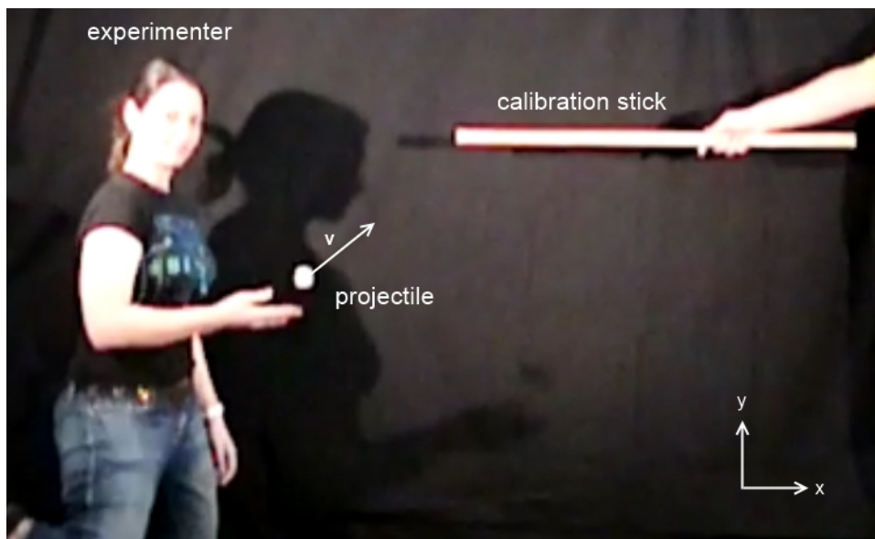
FIG. 1. View of experiment from camera. The experimenter lobbs the projectile with an initial velocity v , such that the ball moves in the x-y plane defined by the coordinate axes. A meter stick placed in the frame allows the computer program to calibrate length. The camera is placed a distance of \sim 2 m from the dark background screen.
