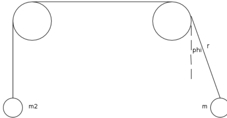
Figure 1: A string connects the two masses in our Swinging Atwood Machine. This string is layed over two pulleys, and the system is allowed to move freely under the force of gravity. One bob of mass m_2 is free to move vertically, while the other bob of mass m is allowed to move radially and tangentially from the point where the string touches the pulley. Phi ( \phi ) is defined as the angle between the string and the vertical, while r is the distance between m and the pulley. We assume massless and frictionless pulleys, as well as a massless and non-extendable string.
