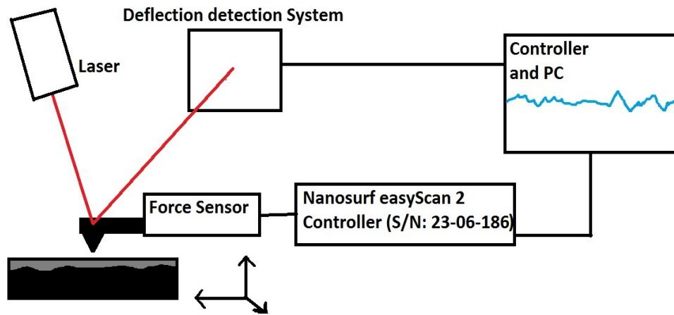
Start up the easyScan 2 or a similar program that is used with the AFM. Be sure to load proper parameters otherwise the images produced will not come out clear. Be sure to ground the AFM sample mount if that option is available. Wear gloves when necessary. Also make sure the AFM is level before and during the duration of the experiment.
